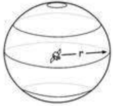
a) with a range measurement from one satellite, the receiver is positioned somewhere on the sphere defined by the satellite position and the range distance, r
